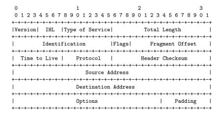
Fig. 2. Structure of IP header according to RFC 791, [14].
