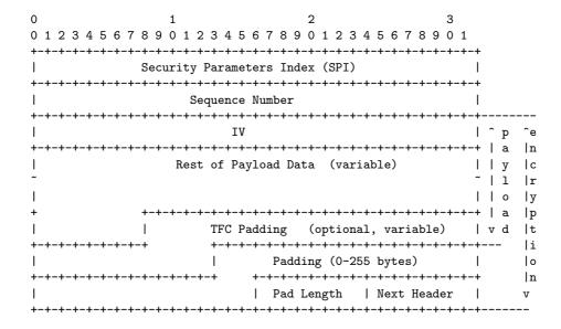
Fig. 1. Structure of ESP protected-datagram (adapted from RFC 4303 [12] for CBC mode without integrity protection and to show encryption scope).
